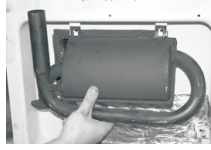
3. Remove Both Mufflers
