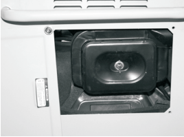
Figure 9 – Changing The Air Filter
