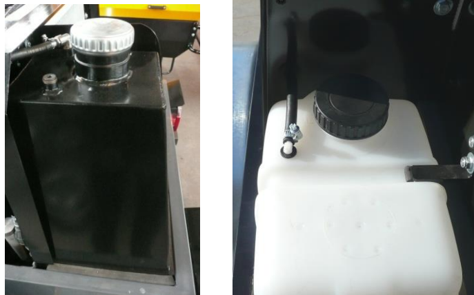
Figure 10.1-2 Gas oil tanks for Diesel engine
