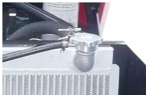
Figure 10.1-3 Checking the radiator cooling liquid
